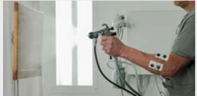
Testing shown involved spraying water during muscle effort monitoring by United States Ergonomics.
